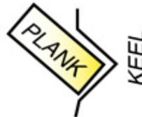
2. Notch rotates in keel to conform to hull shape and keep the plank square in the keel/stem/sternpost rabbet - "L" shape.
